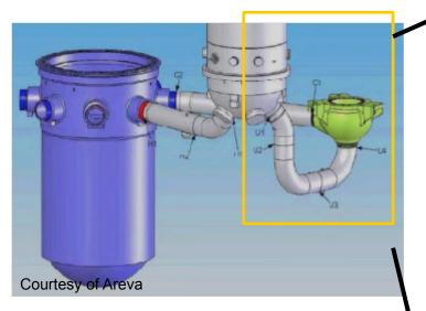
Initial design not optimised for ultrasonic Inspection.
